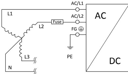
Using a fuse or a circuit break to protect the AC/L2 input is suggested. The AC/L2 input is internally non-protected. Suggested fuse is shown as below.
