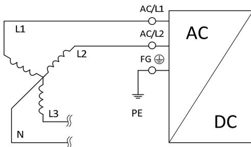
Using a fuse or a circuit break to protect the AC/L2 input is suggested. The AC/L2 input is internally non-protected.
